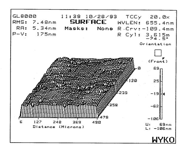
This figure shows surface roughness taken on a WYCO TOPO-3D instrument. This part was ground with an 8000 mesh (1.8 micron diamond) wheel made by the Fuji Die Company. The power supply was a Sintobrator EDM unit modified to output 60 volts and set at 2 microseconds on time and 5 microseconds off time. The ELID dressing current was 0.2 amps. The coolant was Noritake AFG-M at 50:1 dilution with spring water.
