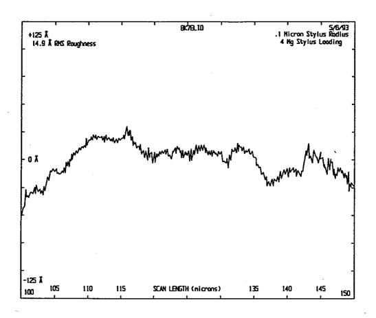
This figure shows 14.9 Angstrom RMS surface roughness taken on a Rank Taylor Hobson Talystep instrument. This is the same part as shown in the previous figure using the 8000 mesh wheel.
