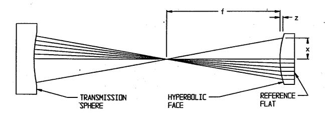
The hyperbola is defined by requiring the axial optical path length of zn + f be equal to the path of the off axis rays as shown:
